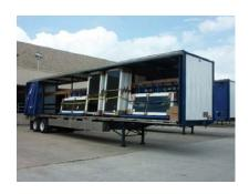
The Delivery System: Experience working in the field gave us the insight to develop a better delivery system. We designed trucks that have a fork lift truck on the back. By using special racks that lock into the truck bed, we can deliver our product on racks directly to the job site or to our dealers' warehouse. This saves time and insures safer handling.
